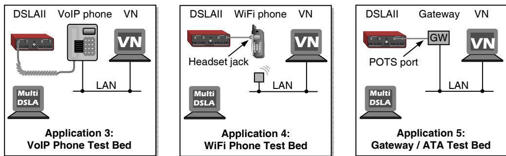
DSLAI provides analogue interfaces; VN provides a digital reference point in a clean network, against which a VoIP terminal or gateway can be tested by developers and Quality Assurance engineers. In all cases the MultiDSLA user interface controls the DSLAI and VN nodes and controls the test process.
