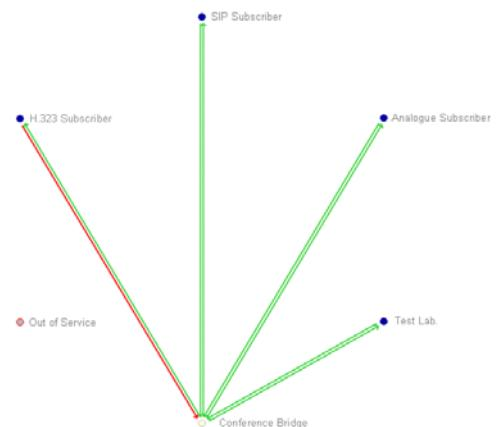
Alternatively, the more complex configuration can be employed in the development laboratory or System Integrator test facility to assess the performance of new designs, software releases or vendors. Evaluation of Conference Bridge performance, simulating many participants with different access networks, is simply achieved in the MultiDSLA user interface. Analysis of results by codec or access network is easily prepared.
